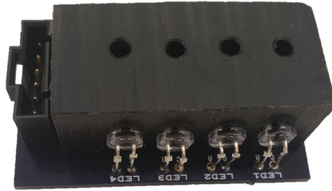
Figure 4: Photoresistor/Diode Solder Detection
